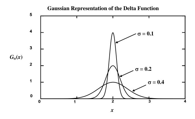
**Question6:** Consider a Gaussian pulse given by  $f t = A e^{-t^2/2\tau^2} e^{-i\omega_0 t}$ . Calculate its frequency spectrum and show that  $\tau \Delta \omega \approx 1$ .
